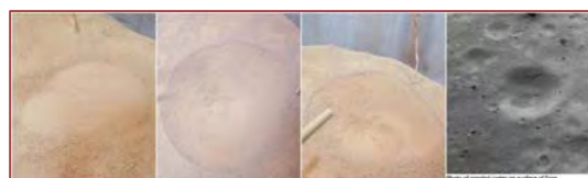
Fig. 6 Pondered craters resulting from loss of water compared with a pondered crater on Eros.
