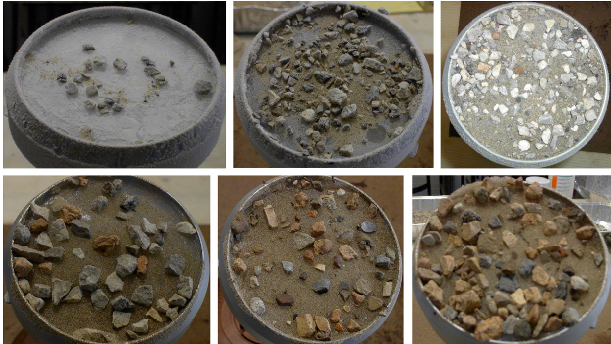
Fig. 3. The surface of the collector after sample collection. (Top left) –75 °C, (top middle) –50 °C, (top right) –25 °C, (bottom left) 23 °C, (bottom middle) 65 °C, (bottom right) 105 °C. Notice the frost on the samples below freezing and the small amount of substrate that flowed in the oven of the 105 °C sample; however, the substrate remained intact and still collected ample sample.
