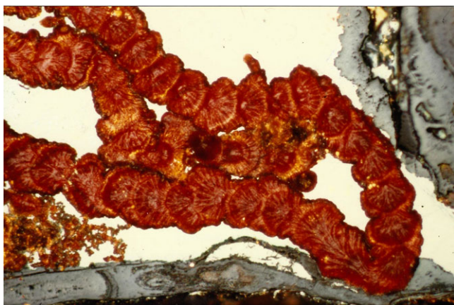
Fig. 7. The Ballinger, Texas, meteorite showing corrosion attack on a polished surface, exposed 24 h in an indoor environment. The orange, circular steps are about 0.2 mm in diameter and contain 2–5% chlorine (Page 522 in Buchwald 2008). (see online version for color figure.)
