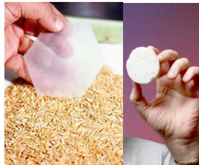
Plastic film prepared from rice hull ash silica
