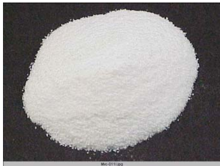
Silica gel produced from rice hull ash
