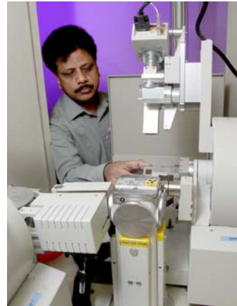
X-ray diffraction to observe ash quality and material structure
