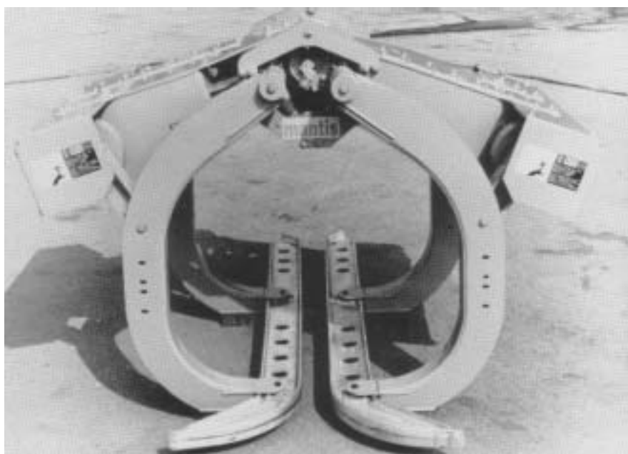
Figure 3. The trunk shaker tits inside an over-the-row harvester and works best on bilateral cordon-trained, spur-pruned vines where each vine is individually staked.
