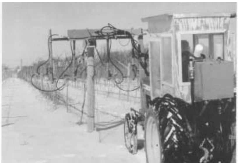
Figure 4. This photo shows a Slawson Mead pruner operating in a research vineyard at the University of Arkansas on a Bilateral Cordon trained system that has been mechanically shoot positioned.
