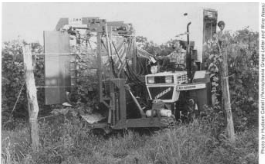
Figure 2. The CMH Harvester, a side-mounted over-the-row unit, was developed in 1976 by the CMH Manufacturing Company in North East, Pennsylvania.
