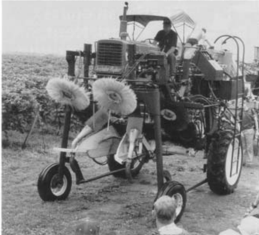
Figure 5. The Oldridge unit is mounted under a Chisholm-Ryder harvester that is designed to position Double Curtain vineyards. Photo taken at Roy Orton's vineyard, Ripley, NY.
