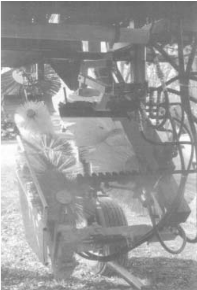
Figure 3. View of the Oldridge shoot positioner in Figure 2 with cutter bars installed for pruning. Brushes pull canes into position to be cut. Both machines are being evaluated at the U of A as well as in other grape-producing regions of the United States.
