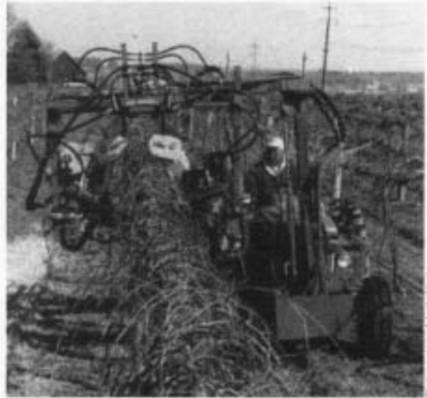
This mechanical pruner is part of the Morris-Oldridge Plan and is used to establish test plots in a bilateral cordon vineyard at the University of Arkansas vineyards.
