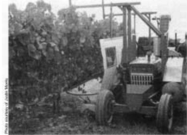
This Lyre or "U" harvester was developed for the Morris-Oldridge Plan and will also harvest the conventional vertical shoot position trellis system. Preliminary results indicate that this unit will harvest a high percentage of whole berries.
